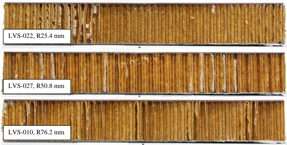
Figure 3.6.5. Cross section of tests LVS-022, 027, and 010 impacted at 4 J with increasing tip radii
