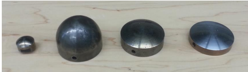
Figure 2.1.2. Impact tips of radii 12.7, 25.4, 50.8, and 76.2 mm (left to right)
