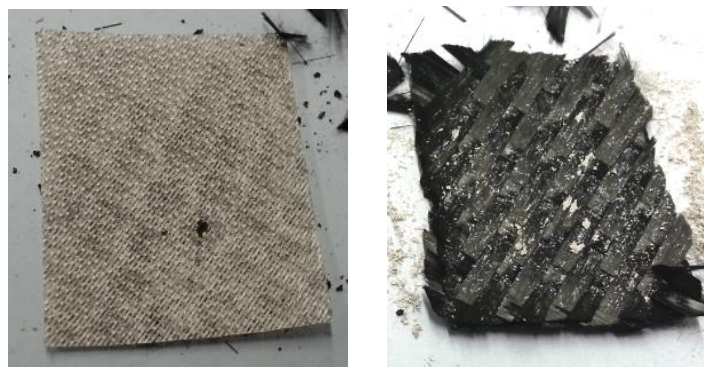
Figure 2.2.2. Inner fiberglass layer (L) and outer carbon fiber layer (R) of top and bottom facesheets
