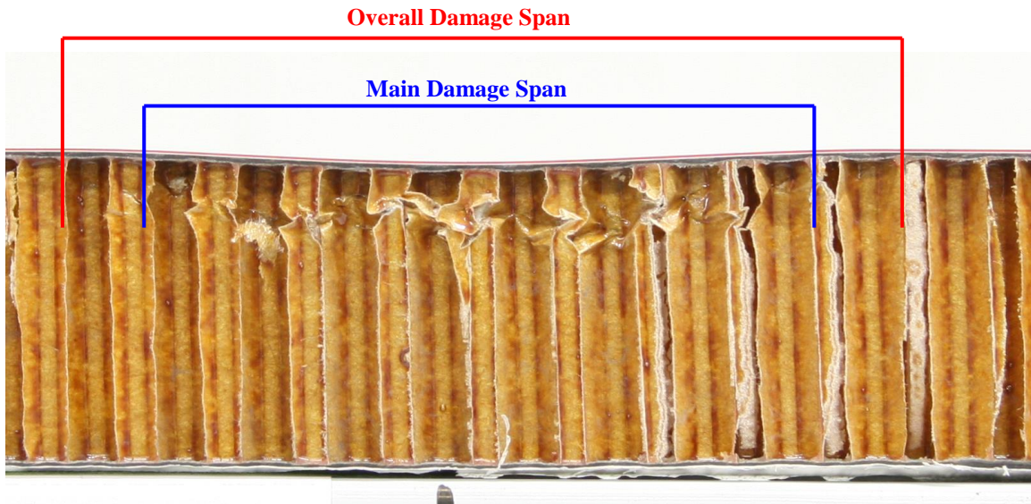
Figure 3.7.1. Overall and main internal damage span
