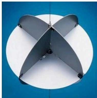
Figure 4.3 Davis Instruments Echomaster™ Radar reflector. Three perpendicular aluminum plane forms 8 corner reflectors.
