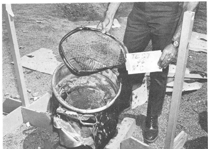
Figure 7. Carrying cask after detonation of 1/4-pound charge.
