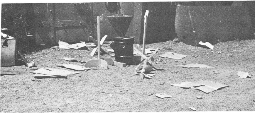
Figure 5. Blast effects of 1/4-pound charge.
