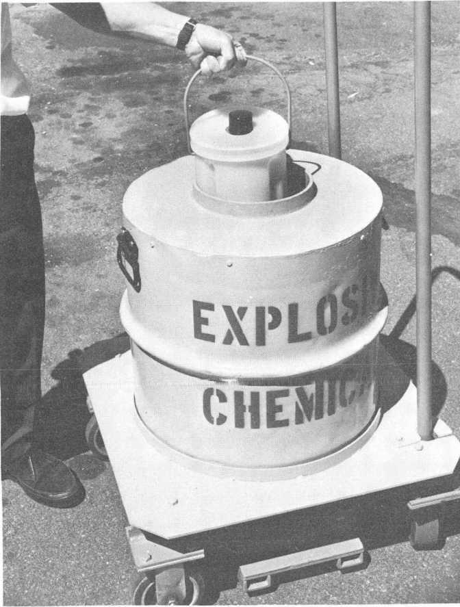
Figure 20. Carrying bucket containing chemical being placed in container.
