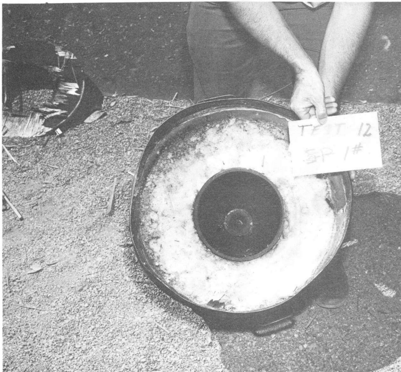
Fig. 12. Polyfoam unit after detonation of 1-pound charge.
