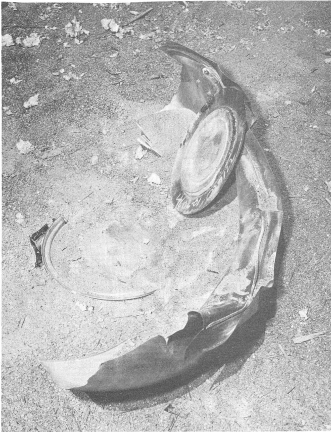
Figure 16. Remains of sand-filled unit.
