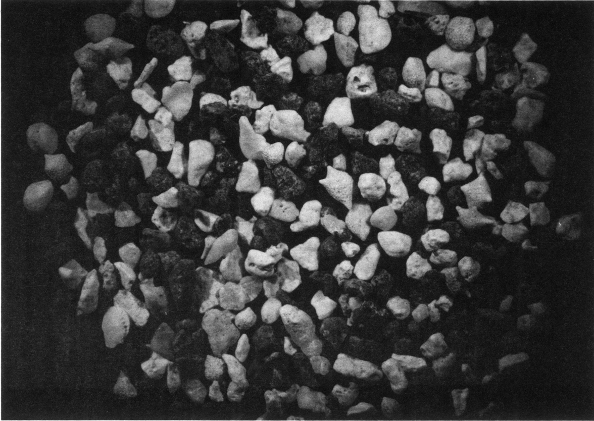
Figure 7.3 Photomicrograph of a typical "salt-and-pepper" sand with mixed calcareous and volcanic-lithic lithology; from Layer IF of Unit 24 (1 phi size fraction; 10X).
