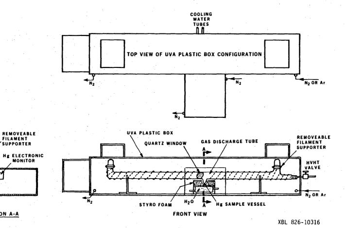
Figure 1. Setup for testing the gas-discharge tube.
