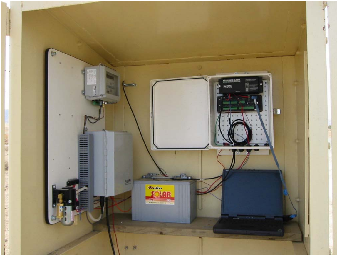
Figure 9. Suggested interior configuration of Design Analysis 350XL and 355 bubbler stage sensor (on left) and the Campbell CR-10X datalogger and associated sensors in center-right.
