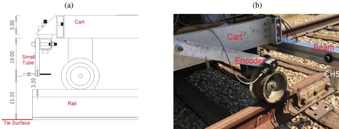
Figure 2.3: (a) Key dimensions of the prototype (unit: inch): the camera is placed ~11.5" above the tie's surface, with a clearance of ~3.5" from the top surface of the rail. (b) Encoder: the transducers and sensors are triggered by an encoder with 0.25" resolution.
