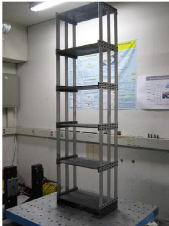
Figure 3.2: Experimental setup of the five-story shear building structure on the shake table.
