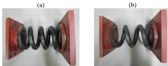
Figure 3.17: Spring members utilized in fabricating the (a) intact and (b) damaged structures.
