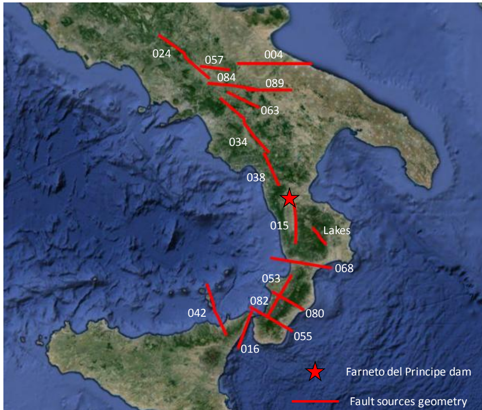
Figure 4.4 Fault sources (finite faults) used in this study.
