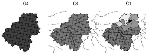
Fig. 2. (a) HRAP coverage over the basin (b) Delineated river and sub-basins (c) Delineated sub-sub-basins. Different gray scales show the contributing area for each river reach.
