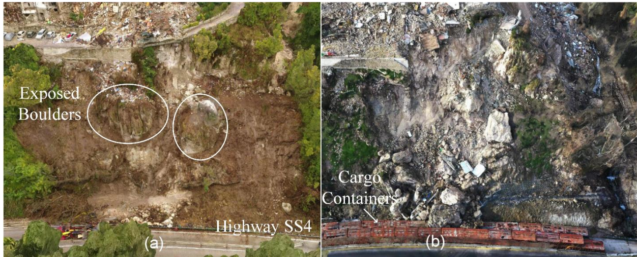
Figure 8. 3D mesh model images of the largest observed debris slide below the village of Pescara del Tronto (a) following the August 24 th event, and (b) following the October 30 th event
