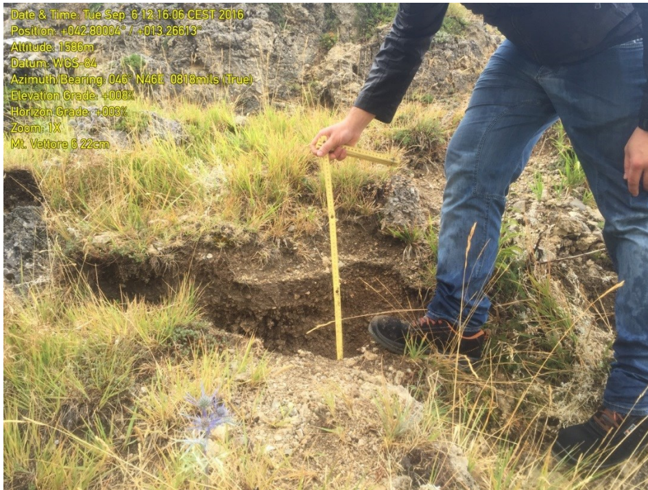
Figure 2.19h. Mt. Vettore fault Site 6 at a WGS84 ellipsoid elevation of 1527 m. The normal fault displacement at this site was 22 cm down toward the west (Latitude and Longitude are annotated on the image).
