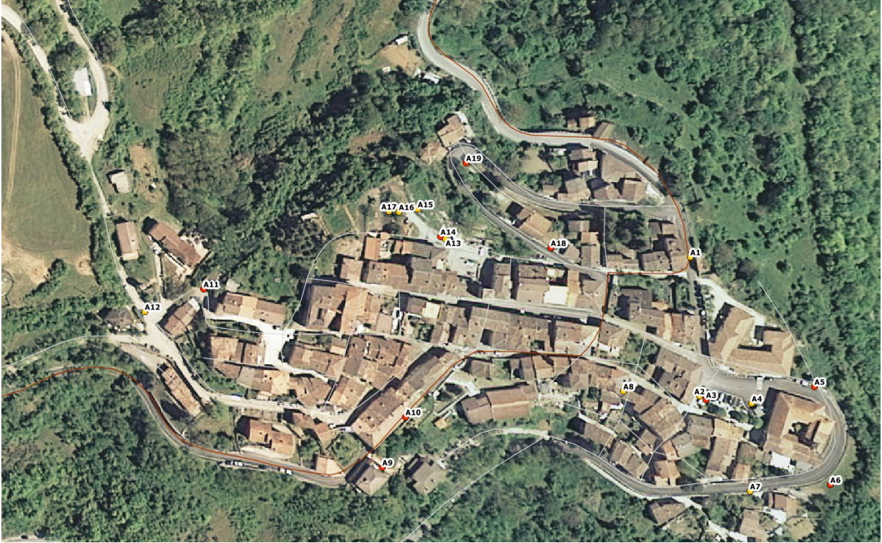
Figure 4.14. Position of the GCPs in Accumoli (red indicates artificial marker, green indicates natural marker).
