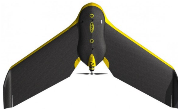
Figure 4.9. The eBee™ small UAV by Sensefly.
