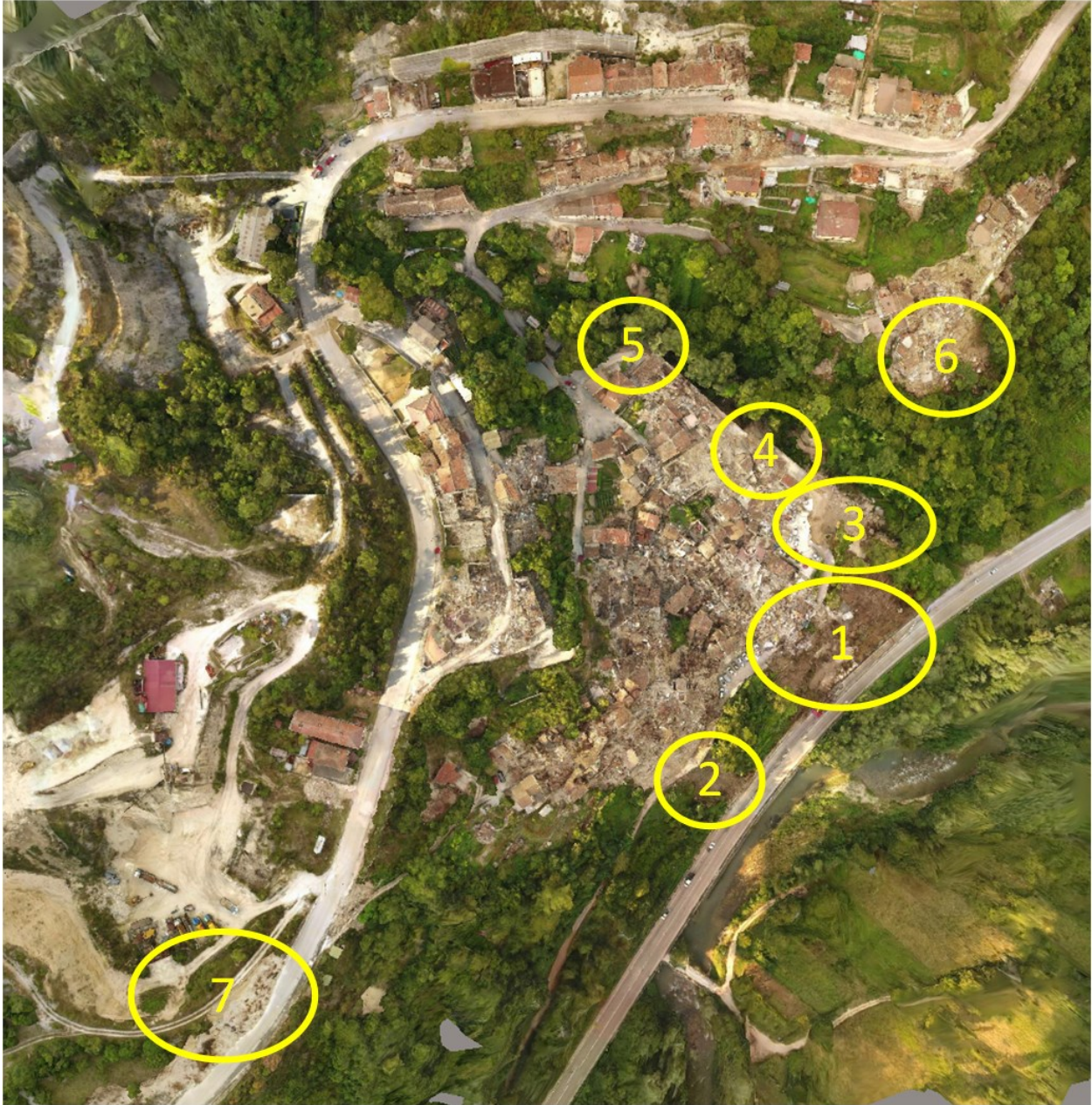
Figure 4.24. Site vicinity map showing the locations of the identified earthquake-induced landslides in Pescara del Tronto
