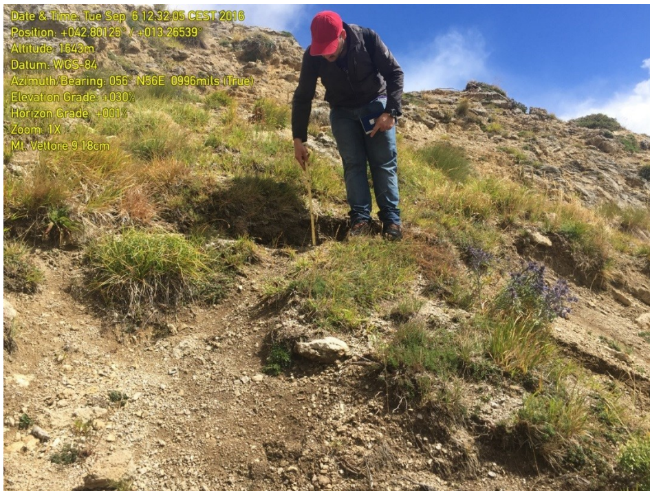
Figure 2.19l. Mt. Vettore fault Site 9 at a WGS84 ellipsoid elevation of 1643 m. The normal fault displacement at this site was 18 cm down toward the west (Latitude and Longitude are annotated on the image).
