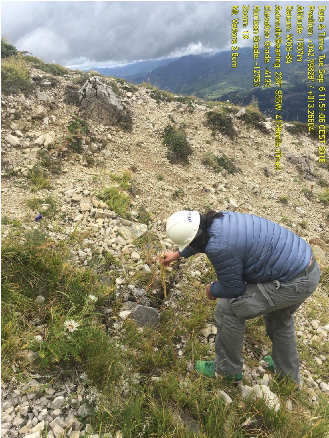
Figure 2.19d. t. Vettore fault Site 2 at a WGS84 ellipsoid elevation of 1507m. The normal fault displacement at this site was 8 cm down toward the west (Latitude and Longitude are annotated on the image).
