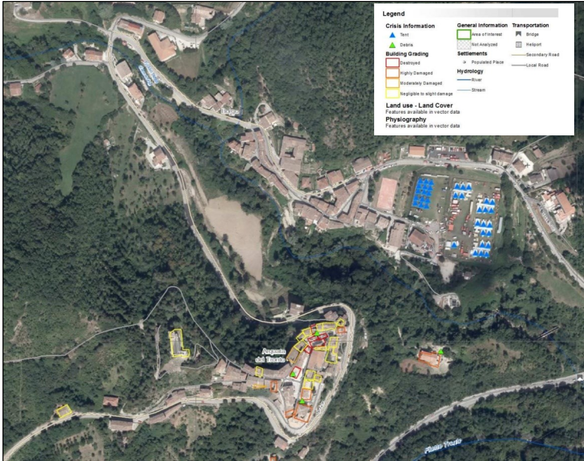
Figure 5.20. Damage pattern from Copernicus post event images ( http://emergency.copernicus.eu/mapping/list-of-components/EMSR177/ALL/EMSR177_19ARQUATADELTRONTOAERIAL )
