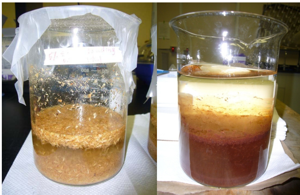
Figure 3.2. Left: Mixture containing 5 wt% maple wood chips in dilute acid water solution, used for non-solvent control reactions. Right: Same biomass slurry mixture with added MIBK extracting solvent on a 1:1 mass basis with the aqueous layer.
