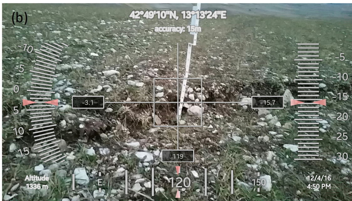
Figure 4. Pictures of the Piano Grande fault offset location; (a) surface rupture manifestation on the road, and (b) rupture manifestation with vertical offset equal to 15 cm.
