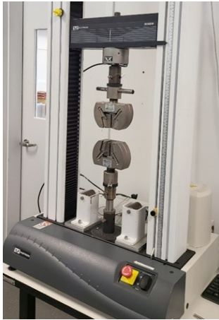
Figure 5: INSTRON 3369 universal testing machine equipped for tensile testing
