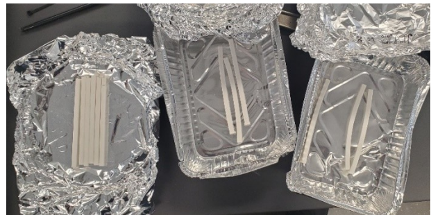
Figure 4: PLA samples: the control samples (left) versus the rapidly cooled (center) and slow cooled (right) heat-treated samples
