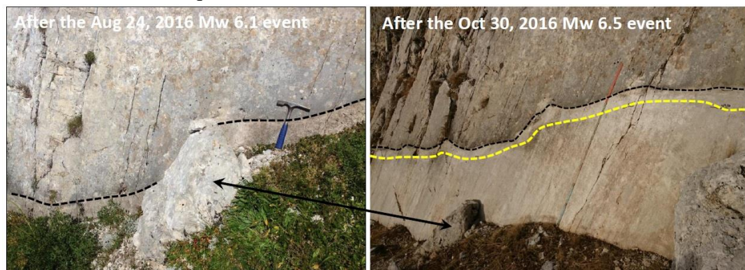
Figure 3. Comparative fault offset between the M6.1 24 August event (left picture) and the M6.5 30 October event (right picture).
