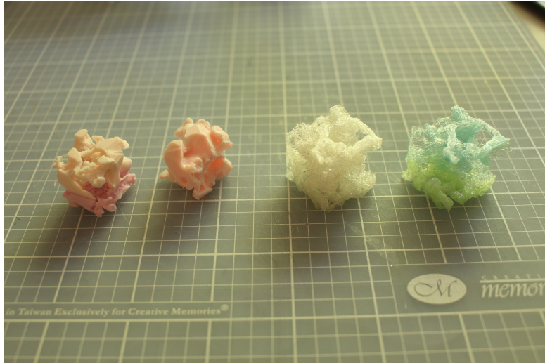
Figure 5.2: Less optimal results from screened Poisson reconstruction (left) versus Marching Cubes (right). Various colors, PLA, .16-.24 layer heights, no supports.
